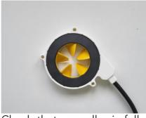
Check that propeller is fully seated and rings are parallel. Manually rotate rings to check for free movement.
