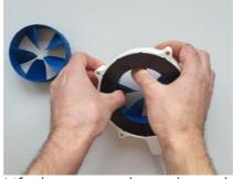
Lift thruster and gently push down against two propeller blades near the outer ring until bottom ring falls out.
