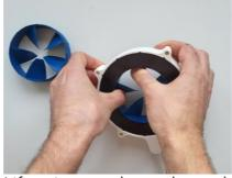
Lift mixer and gently push down against two propeller blades near the outer ring until bottom ring falls out.
