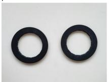
Remove old propeller. Check that magnet rings are clean.
